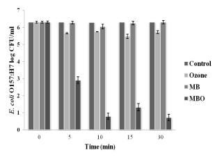
Figure 4. Effect of micro-bubbles ozone in water at 13°C on growth inhibition of *E. coli* O157:H7 after incubated for 48 h.\*Error bar represented standard deviations. Values (log CFU/ml) with the same letter on the same color bars represented no significance differences (\*P>0.05)
