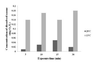
Figure 2. Concentrations of dissolved ozone in water was measured by Indigo colorimetric method at 28 and 13°C
